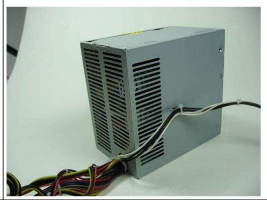
3. Remove the four power supply chassis screws—two from each side.
