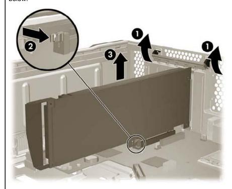
Release the card slot latch (2, and then carefully lift the card from the chassis (3).
