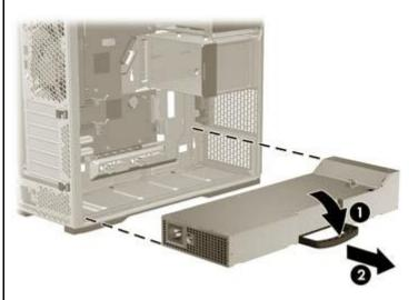
Use the handle to pull the power supply out of the chassis 2.
