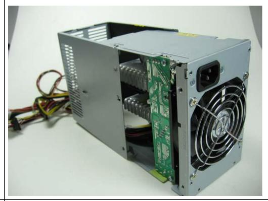
Remove the four screws from the corners of the large PCB card. Remove the large PCB card from the unit.
