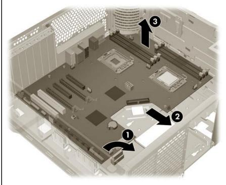
Slide the system board forward 2, and lift it from the chassis 3.
