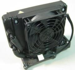
3. Drain the coolant from the closed loop system. This is done by cutting the tubes, as shown in the following two pictures.
