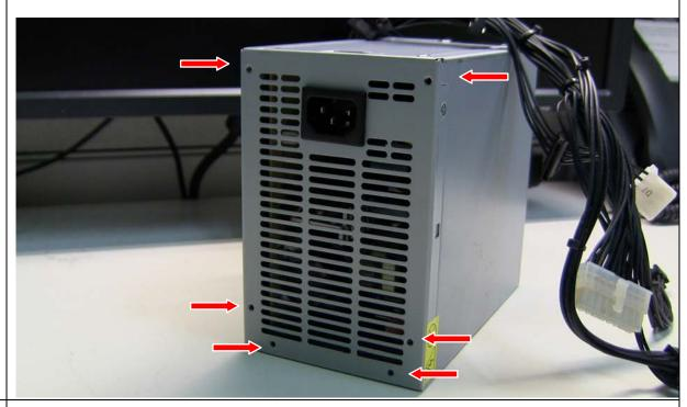
3. Slide the chassis housing from the power supply unit.
