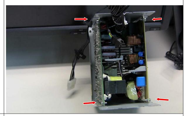
5. Ensure that all capacitors are safely discharged. Use a diagonal cutter to remove the desired components from the PCA. (Note that some components may need to be unsoldered if a diagonal cutter does not fit between the component and the PCA.)
