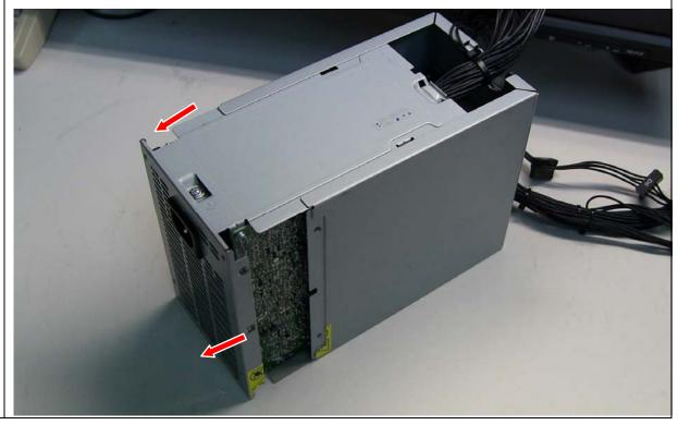
4. Remove all screws from the corners of the power unit. The unit opens into two parts.
