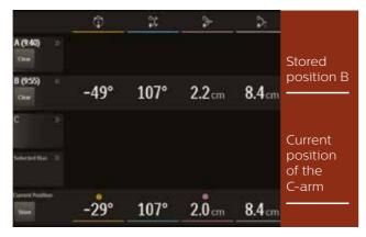
Position Memory stores a previous position and displays it on the monitor above the current position of the C-arm, helping the user quickly return to the desired view with accuracy.
