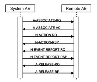
Figure 7: (Real World) Activity – Synchronous Storage Commitment Push Model as SCU within one association (synchronous)
