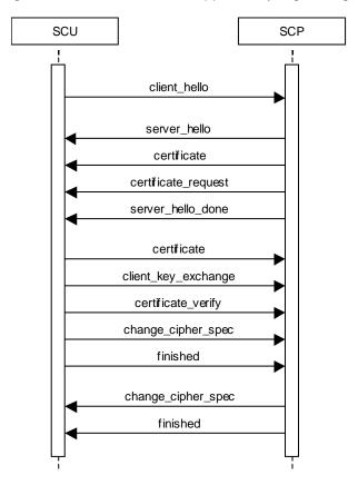
Figure 15 Message flow of TLS handshake
