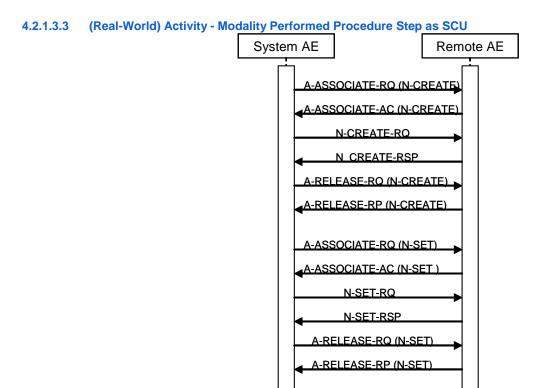
Figure 8 (Real World) Activity - Modality Performed Procedure Step as SCU
