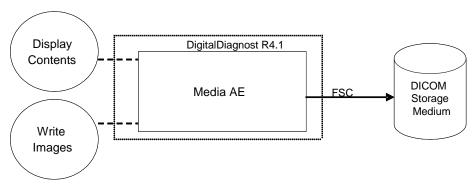
Figure 14: Media Interchange Application Data Flow Diagram
