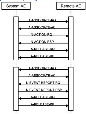
Figure 6: (Real World) Activity - Storage Commitment Push Model as SCU within separate associations (asynchronous)
