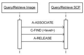
Figure 4 Data Flow Diagram - FIND as SCU
