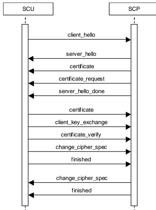
Figure 14: Message flow of TLS handshake
