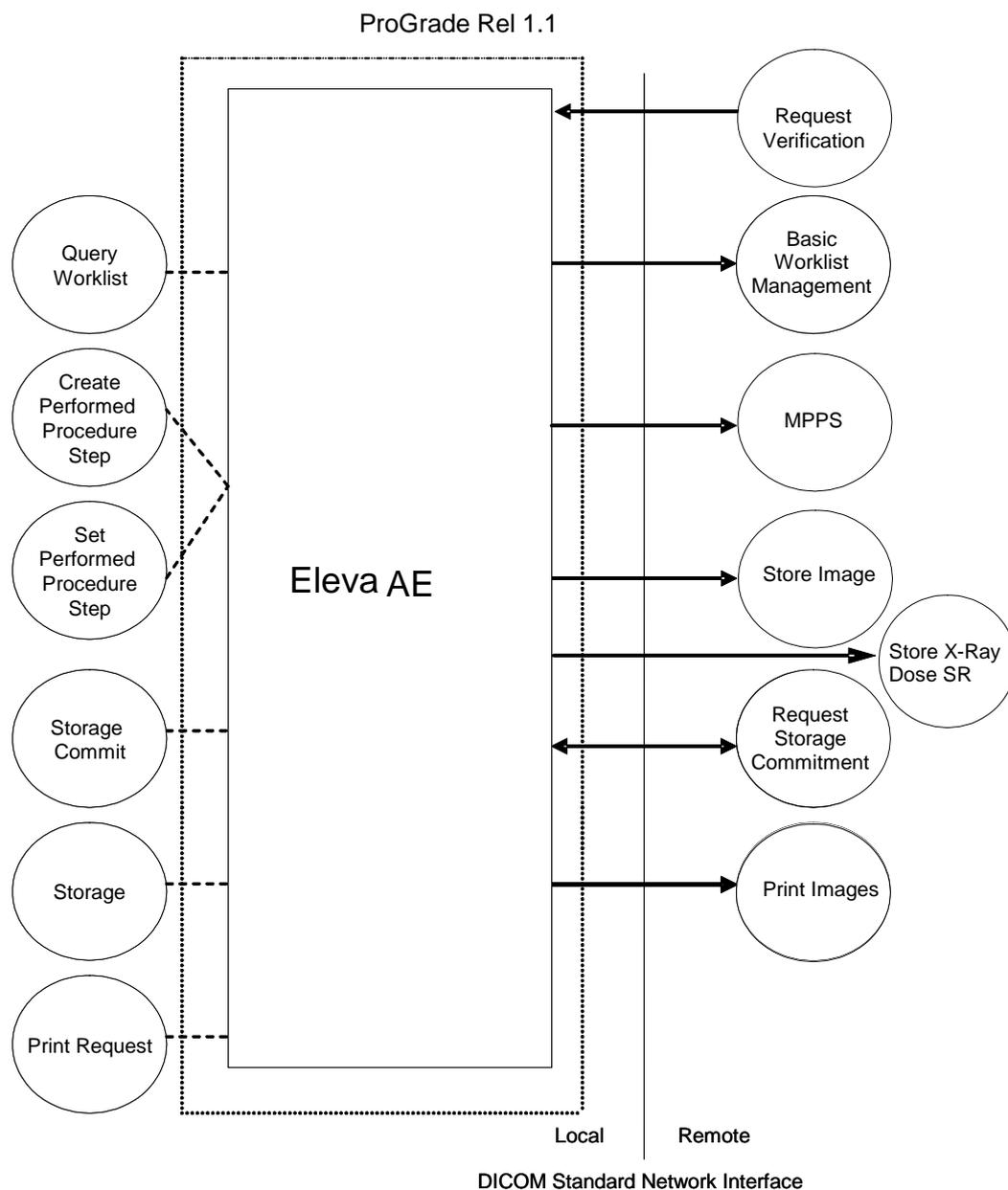
**Figure 2: Application Data Flow Diagram**
