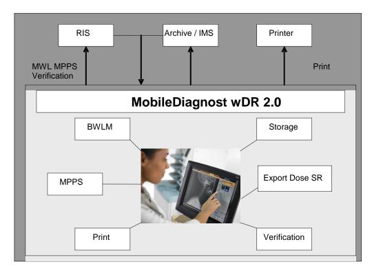
Figure 1: MobileDiagnost wDR 2.0 in a DICOM network
