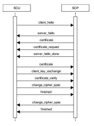
Figure 14: Message flow of TLS handshake
