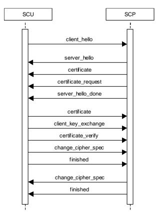
Figure 13: Message flow of TLS handshake
