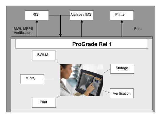
Figure 1: ProGrade Rel 1 in a DICOM network
