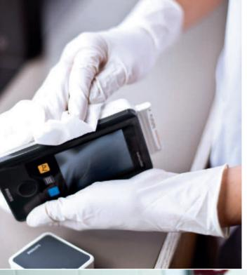
The IntelliVue MX40 is protected against the effects of temporary immersion in water (to IPX7) and able to withstand showering, cleaning, and periodic sterilization.
