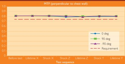
To demonstrate that MicroDose Mammography could maintain performance and reliability despite the rigors of travel, a system was mounted onto a vibration testing platform and subjected to lifetime testing. The graph demonstrates the consistency maintained during these tests.
