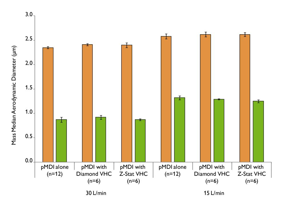
Figure 5. Mean Mass Median Aerodynamic Diameter (MMAD) of the aerosol from the pMDI alone, pMDI with Diamond VHC and pMDI with Z-Stat VHC for albuterol 🗖 and ipratropium bromide 🔲. Error bars denote standard deviation about the mean.
