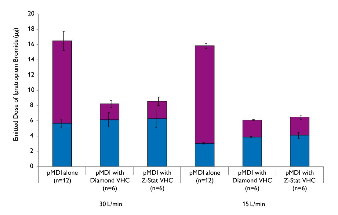
Figure 4. Emitted dose (drug entering the NGI) from the pMDI alone, pMDI with Diamond VHC and pMDI with Z-Stat VHC using ipratropium bromide. Fine particle dose is highlighted and the dose in particles > 4.7 µm highlighted . Error bars denote standard deviation about the mean.
