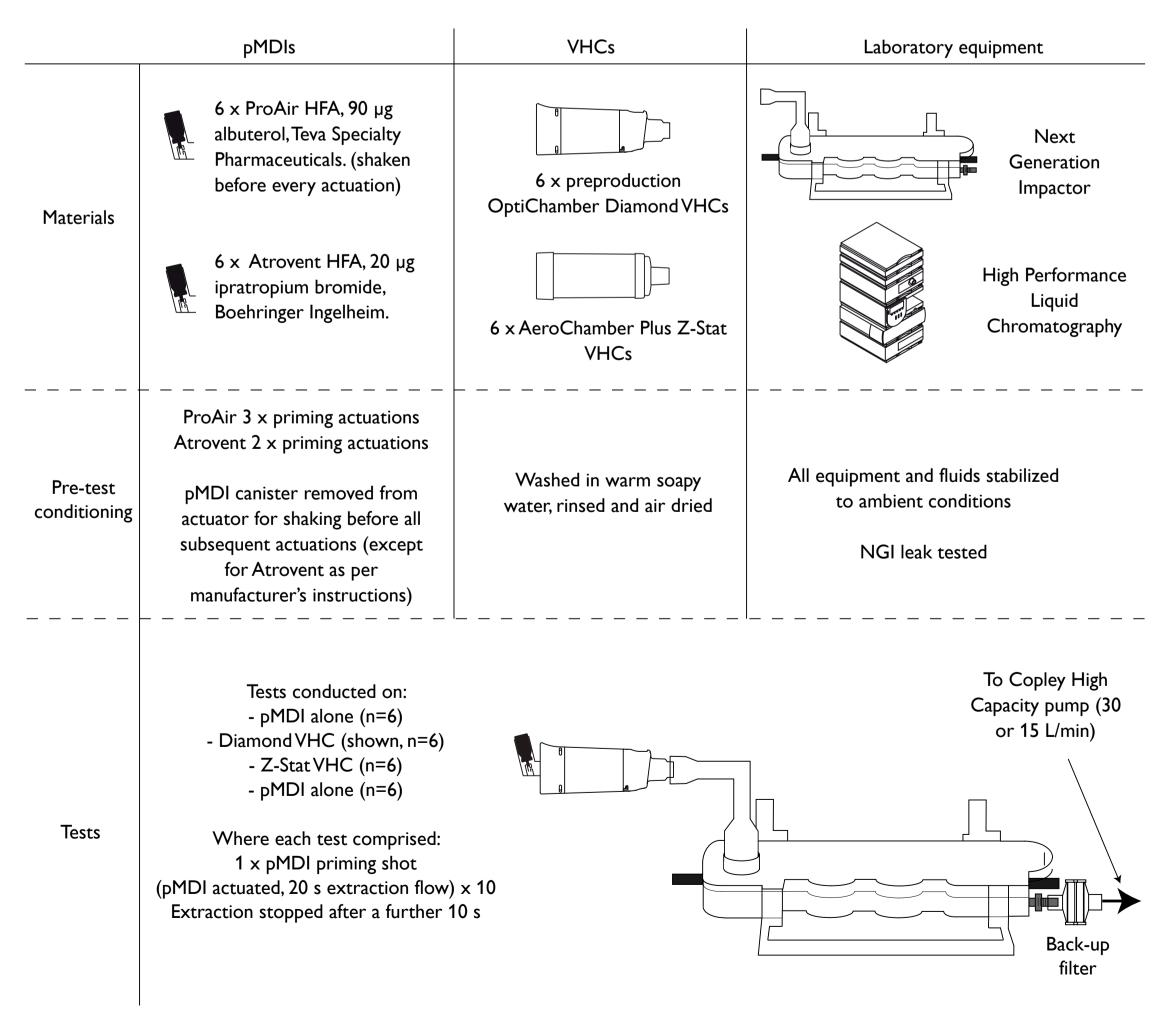
After each test the induction port, back-up filter, NGI cups and VHCs were processed using HPLC assay diluent for ipratropium bromide tests and 10% acetonitrile solution for albuterol tests. CITDAS V3.10 software was used to generate the aerosol characteristics data. The mean emitted dose (drug entering NGI), fine particle dose (amount of drug in NGI  $\leq$  4.7 µm), and Mass Median Aerodynamic Diameter (MMAD) were calculated. The equipment was washed and dried after each drug/VHC test.
