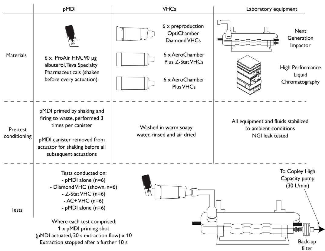
Figure 2. Experimental test method.
