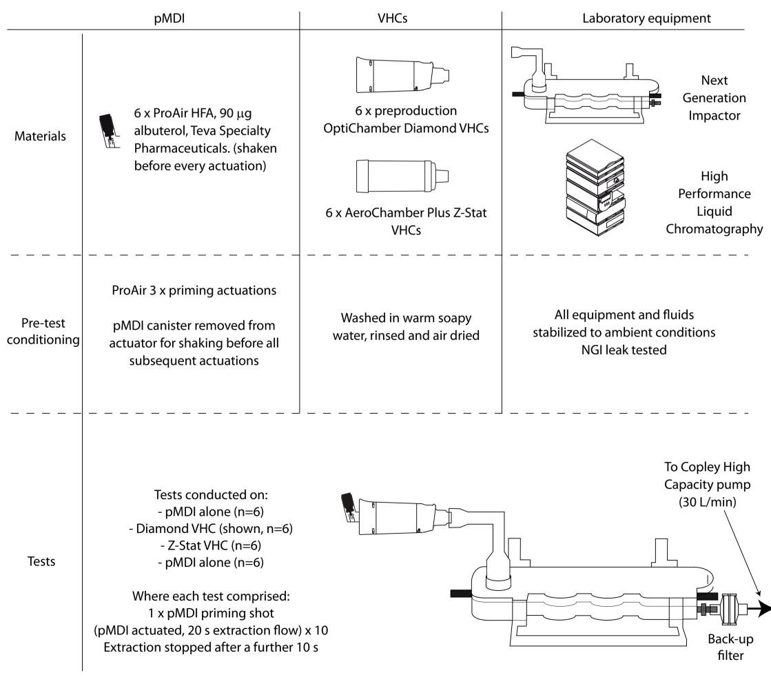
Figure 2. Experimental test method.
