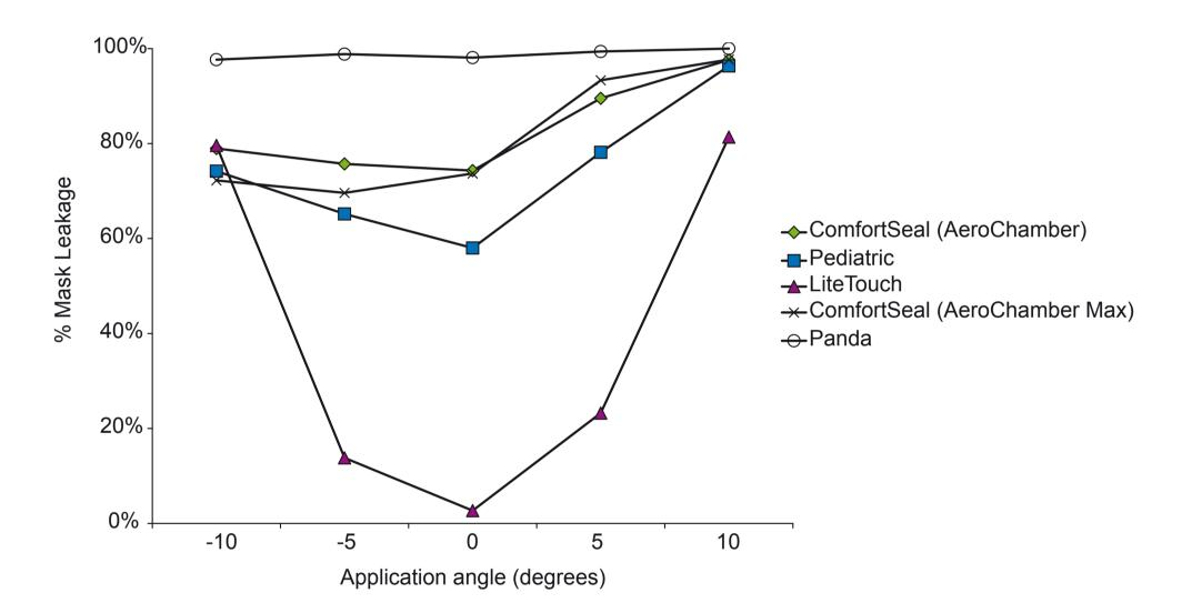
Figure 2. Effect of application angle on leak between face and facemask with 0.45 kg applied force.
