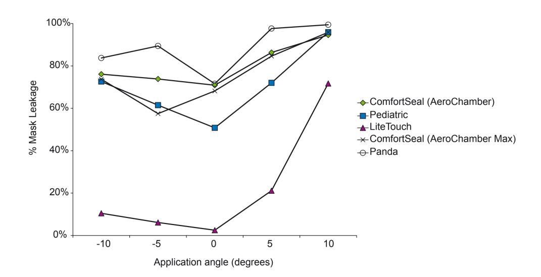
Figure 3. Effect of application angle on leak between face and facemask with 0.9 kg applied force.
