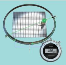
Astonish TF Time-of-Flight technology uses the actual time difference between the detection of coincident events to more accurately identify the origin of the annihilation. TOF reduces noise during the image acquisition, improving the information sent to reconstruction and leading to detectability of small lesions, reduced dose, and rapid scan times.
