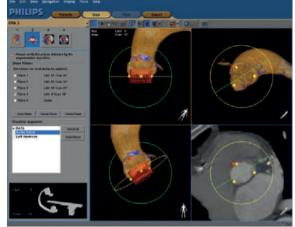
**Step 4. Live overlay image.** During the procedure, you can use the 3D reference image on the normal monitor and the 3D live overlay on the X-ray image to get real-time feedback as you navigate through vasculature. The overlay automatically follows the C-arm position and all system movements can be controlled at tableside.
