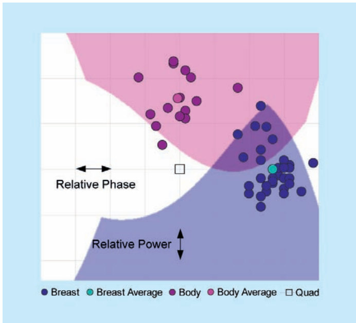
Figure 4 Patient-adaptive shimming - typical distribution of RF shim settings.
