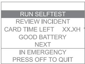
To run the battery insertion selftest, remove and reinstall the battery. The screen tells you whether or not a data card is installed. If it is, a screen message displays how much recording time is left until the data card is full.
