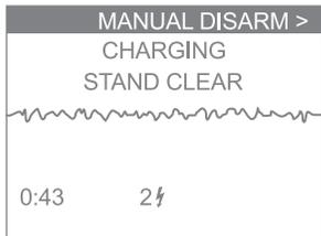
As soon as charging begins, the screen message changes to **CHARGING**, **STAND CLEAR**, and the label for the arrowhead pointing to the upper Option button changes to **MANUAL DISARM**.
