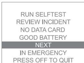
1. Remove and reinstall the battery of both FR2+ devices to bring up the first menu screen.
