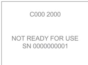
Replace the battery with a new battery and repeat the test. If the second selftest fails, contact Philips for technical support.
