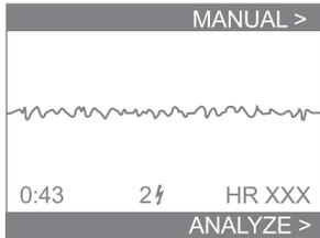
To enter the advanced mode during use of an FR2+ that has this feature enabled, make sure pads are attached to the patient, then press both Option buttons simultaneously. This brings up a screen that includes a highlighted line at the top, labeled **MANUAL**, with an arrowhead pointing to the upper Option button, and another at the bottom, labeled **ANALYZE**, with an arrowhead pointing to the lower Option button.
