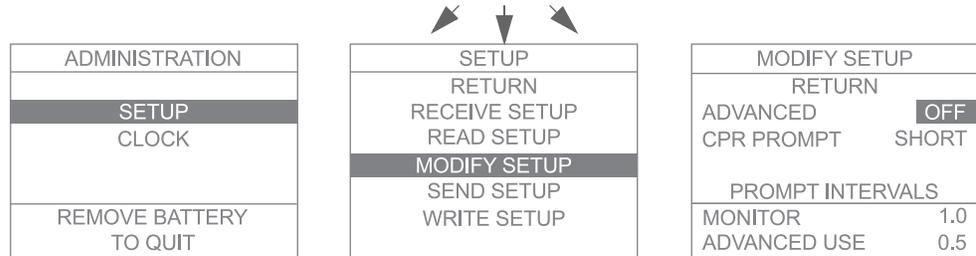
Using the upper Option button, scroll through the available settings for ADVANCED. The advanced mode options available are based on the FR2+ model used. For the M3860A, the user can select ANALYZE, CHARGE, or OFF. For the M3861A the user can select only ANALYZE or OFF. (Detailed directions for use are supplied with the Training & Administration Pack.)
