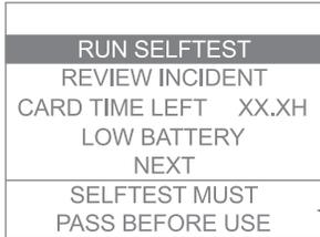
**NOTE:**The data card is typically capable of storing a number of incidents. However, it is recommended that it be cleared or replaced after every use. In the unlikely event that the card fills up during an incident, no further data can be recorded, so it is important for you to monitor the CARD TIME LEFT information on this screen.
