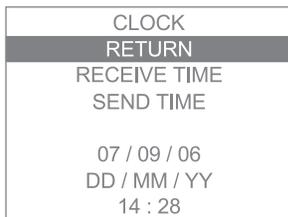
8. Use the lower Option button to move to any other date or time field to be changed, and repeat step 6.
