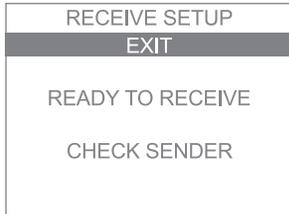
4. A new screen comes up. Until the two HeartStart FR2+ devices are properly positioned, the screen displays READY TO RECEIVE and prompts you to check the sending FR2+.
