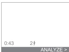
To enter the advanced mode during use of an FR2+ that has this feature enabled, make sure pads are attached to the patient, then press both Option buttons simultaneously. This brings up a screen that includes a highlighted line at the bottom, labeled ANALYZE, with an arrowhead pointing to the lower Option button.
