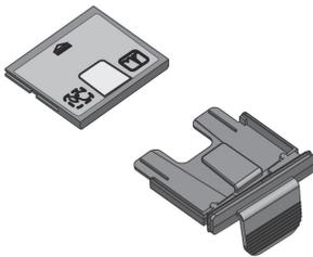
1. Load the data card face up into the data card tray, with the tray's "tongue" fitting over the matching yellow area on the data card.
