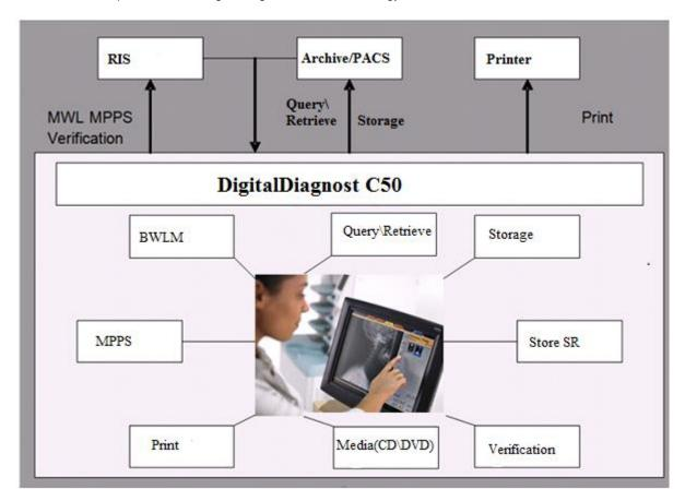
Figure 1 DigitalDiagnost C50 in a DICOM network
