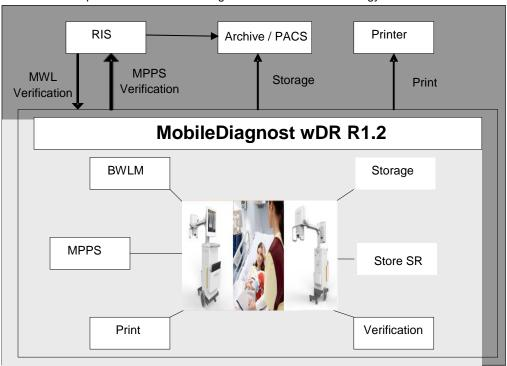
Figure 1 MobileDiagnost wDR R1.2 in a DICOM network
