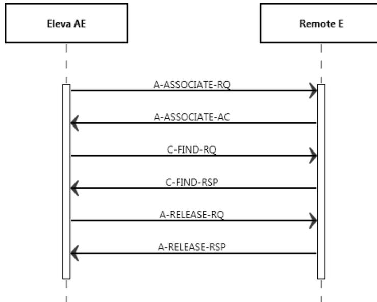
Figure 13: Data Flow Diagram – FIND as SCU
