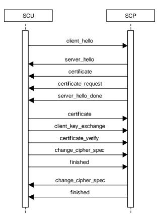
Figure 14 Message flow of TLS handshake
