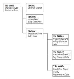
Figure 1 X-Ray Radiation Dose SR IOD Template Structure
