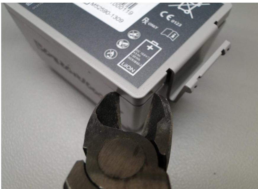
USING SIDE CUTTER TOOL, SNIP EACH CORNER AT WELD LINE (SEAM) – FOUR PLACES
