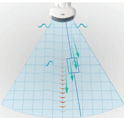
Philips elastography generates shear waves inside the liver by using acoustic force from a focused ultrasound beam. It then monitors shear wave propagation, measures the velocity, and displays results in a format that is easy to interpret.
