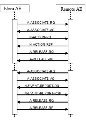
Figure 10: (Real World) Activity – Storage Commitment Push Model as SCU within separate associations (asynchronous)
