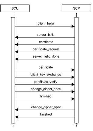
Figure 14: Message flow of TLS handshake
