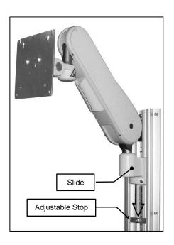
**4.3** Using a 1/8" hex wrench (supplied), tighten (CW) the (2) set screws in the Slide to secure position of Arm.
