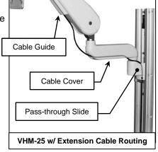
**7.2.3** A "pass-through" channel slide allows cables to run behind the arm within the Channel. **Note:** If cable connectors are too large to fit through the pass-through, try placing the cables in the path of the Slide before installing the arm in the Channel.
