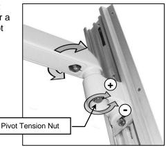
6.5 Center Pivot Tension Adjustment (VHM-25 with Extension)- Insert finger into the front of the Cable Cover and pull down to remove (Fig. A). Tighten (+) or loosen (-) the Pivot Tension Nut with a 3/4" or a 19 mm socket wrench until desired tension is achieved (Fig. B). Push Cable Cover up into the Arm until the tabs on the side of the Cable Cover snap into place (Fig. C). Do not remove the Pivot Tension Nut.
