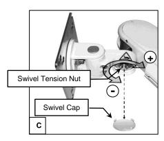
**Rear Pivot Tension Adjustment** – To adjust the tension at the rear Pivot Point (closest to channel), tighten (+) or loosen (-) the Pivot Tension Nut with a 3/4" or a 19 mm socket wrench until desired tension is achieved. Do not remove the Pivot Tension Nut.
