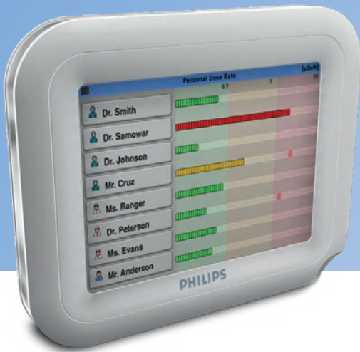
The BaseStation, a LCD touchscreen displays real time dose data for all PDMs within range, to enable you and your staff to take immediate action.
