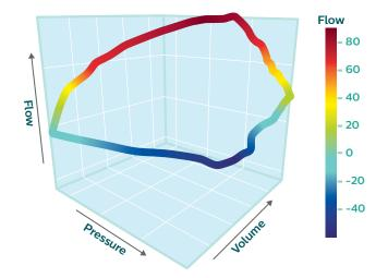
Figure 1 The relationships between flow, pressure and volume (with a mechanical breath from a test lung)
