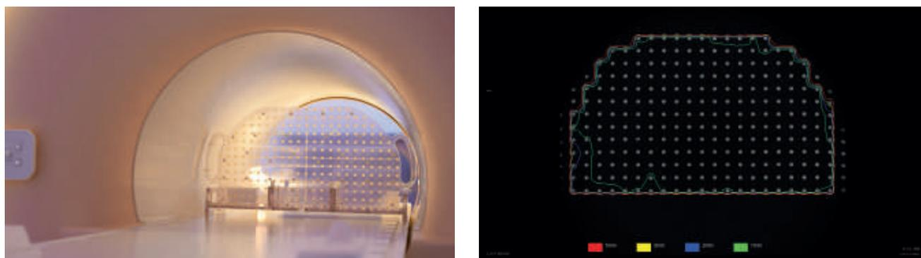
Figure 8. The geometric distortion phantom travels through the magnet’s bore and a scan protocol maps it in 3D in seven parallel volumes. Automated analysis provides accuracy contours. In addition, the phantom can be used to assess the distortion in sagittal and coronal planes.
