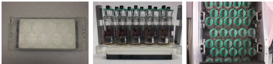
Figure 2 The Astonish TF technology design. The 4 mm x 4 mm x 22 mm LYSO crystals are assembled in a 23 x 44 array and are coupled through a light guide (left) to a hexagonal arrangement of fast PMTs to create a detector module (middle). Multiple modules are assembled in the scanner (right).
