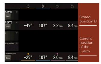
Position Memory stores a previous position and displays it on the monitor above the current position of the C-arm, helping the user quickly return to the desired view with great
