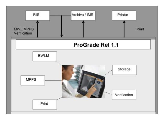
Figure 1: ProGrade Rel 1.1 in a DICOM network
