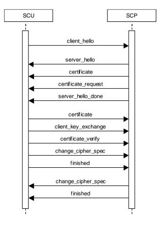
Figure 14: Message flow of TLS handshake
