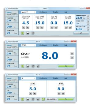
OmniLab Direct allows patient settings and modes to be changed remotely from the control room
