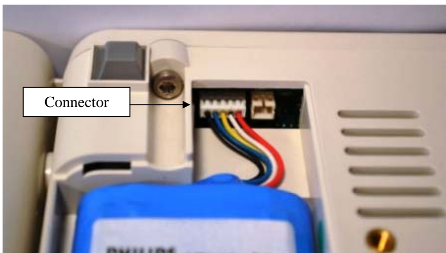
Figure 4 - Disconnect the battery cable from the connector and remove the battery from the monitor
