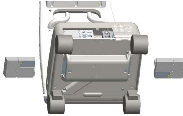
Figure 5: Cart Configuration, Battery Removal
