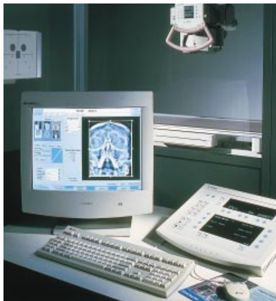
Fig. 2. Digital Diagnost system with integrated flat-panel detector.
