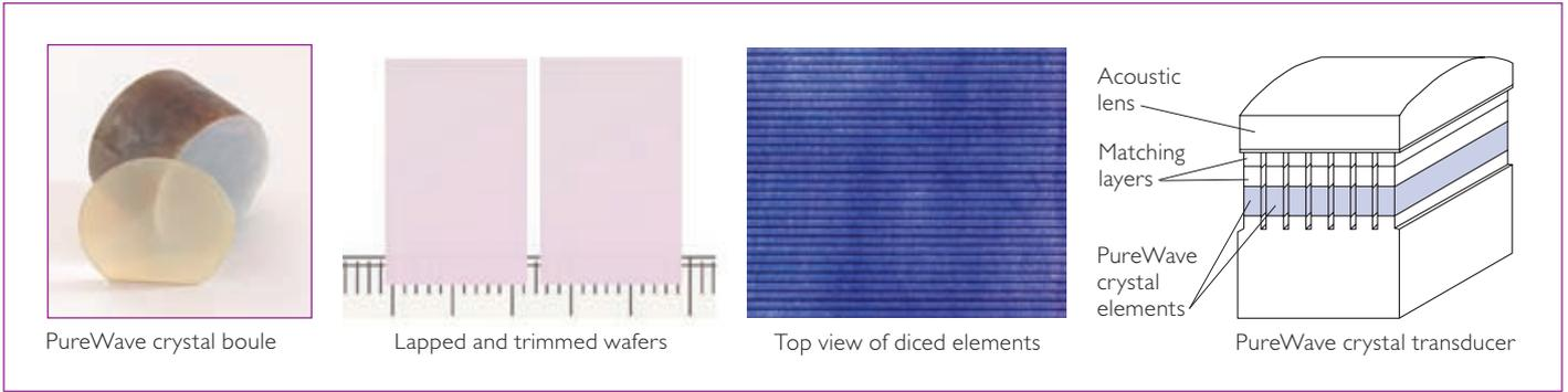
Figure 2. Element manufacture from PureWave crystal boule
