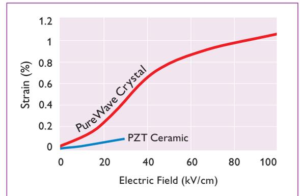
Figure 4. Strain behavior of PureWave crystals vs. traditional PZT-type materials
