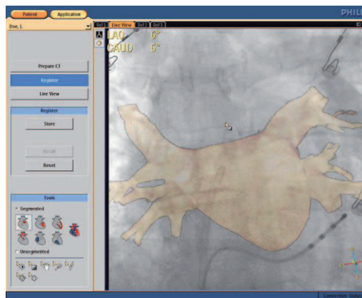
EP navigator shows the position of any catheter with respect to detailed 3D cardiac anatomy in real time.
