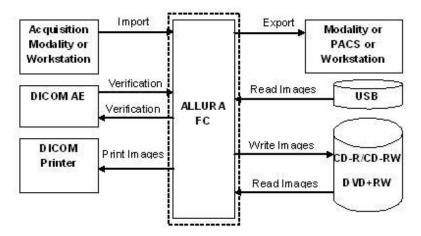
Figure 1: Allura FC System in a DICOM network overview
