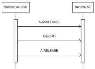
Figure 4: Sequencing of RWA Verification Application Level Communication
