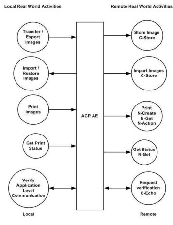
DICOM Standard Interface Figure 2: Application Flow Diagram
