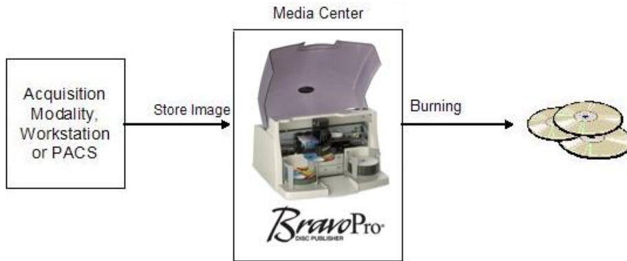
Figure 1: Media Center in a DICOM Network
