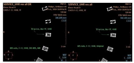
Figure 20: Line-pair phantom demonstrating equivalent spatial-resolution independent of iDose<sup>4</sup> level.
