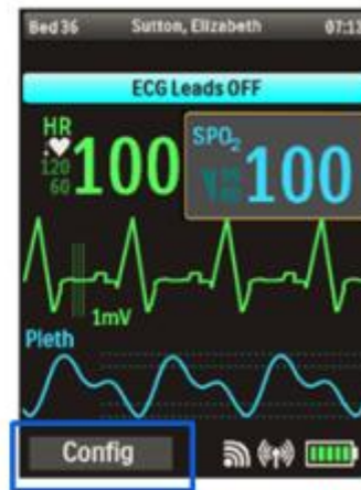
Configuration, Service and Demo mode operation indicated in status area, and on IIC
