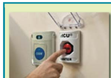
Figure 2 VISICU eLERT button allows staff in the intensive care unit to request the on-camera presence of the tele-ICU team. Both 1-way and 2-way audio/video communications are available for tele-ICU use.
