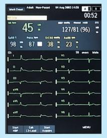
In 12-lead preview mode, 12 waves are viewable on-screen, in addition to numeric vital sign values.
