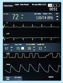
A typical monitoring view shows some basic patient information, the date, time and battery status. Next are the numerics and waveforms. The bottom half of the screen shows additional monitoring numerics followed by their waveforms, and soft keys for customizing the display, setting and responding to alarms, and selecting parameters to view additional monitoring data.
