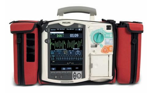
In code view, a single large ECG wave is shown in the top half of the display, the incident timer is prominent and all alarms are paused. CPR numerics and the compression wave appear in the middle. The bottom of the display accomodates the CO2 wave and active soft keys.
