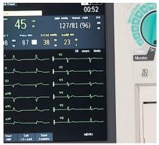
The 8.4-inch color display is well protected against damage. Recessed behind a 3 mm non-reflective polycarbonate shield, framed and backed in an energy-absorbing foam blanket, and supported by a rigid magnesium casting, it endures routine impact from bumps, knocks, and even drops.
