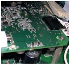
Internal assemblies are rugged. Latched connectors hold cables in place to ensure uninterrupted communications between circuit boards. And every circuit board is aggressively reinforced, braced and fastened at multiple points, keeping the device's internal structure rigid, even in high vibration environments.
