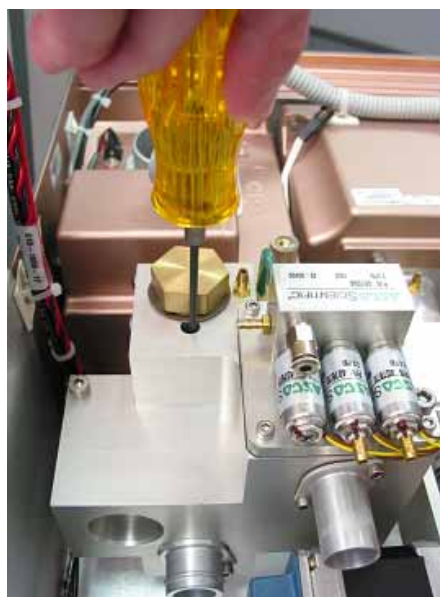
Figure 9-73: Recessed 2.5-mm Set Screw Securing Outlet Port
