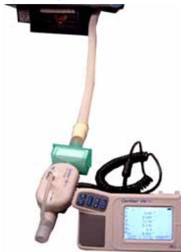
Figure 5-10: Flow Sensor Troubleshooting Setup
