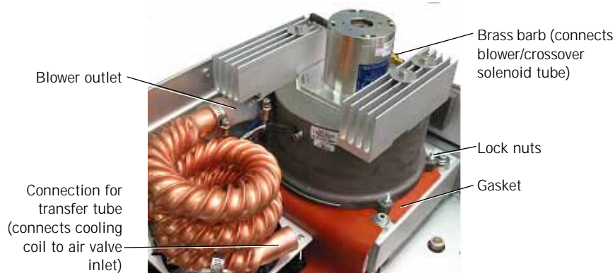
Figure 10-57: Blower Assembly Position on Gasket
