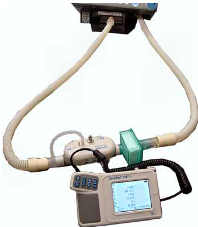
Figure 5-16: Inhalation and Exhalation Pressure Transducer Troubleshooting Setup
