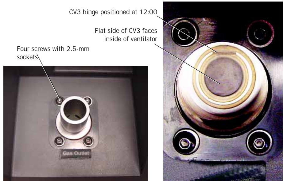
Figure 9-74: Inspiratory Outlet Port and Check Valve CV3 Orientation
