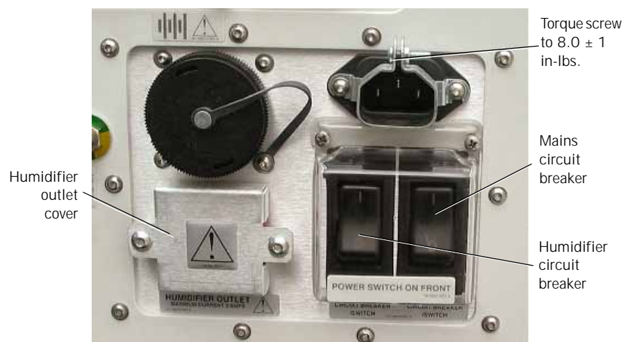
Figure 9-50: Humidifier Outlet Cover
