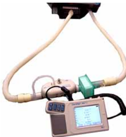
Figure 5-14: Exhalation Flow Sensor Troubleshooting Setup
