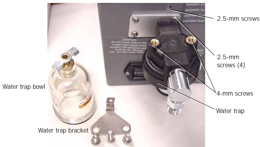
Figure 9-82: Oxygen Water Trap and Oxygen Regulator
