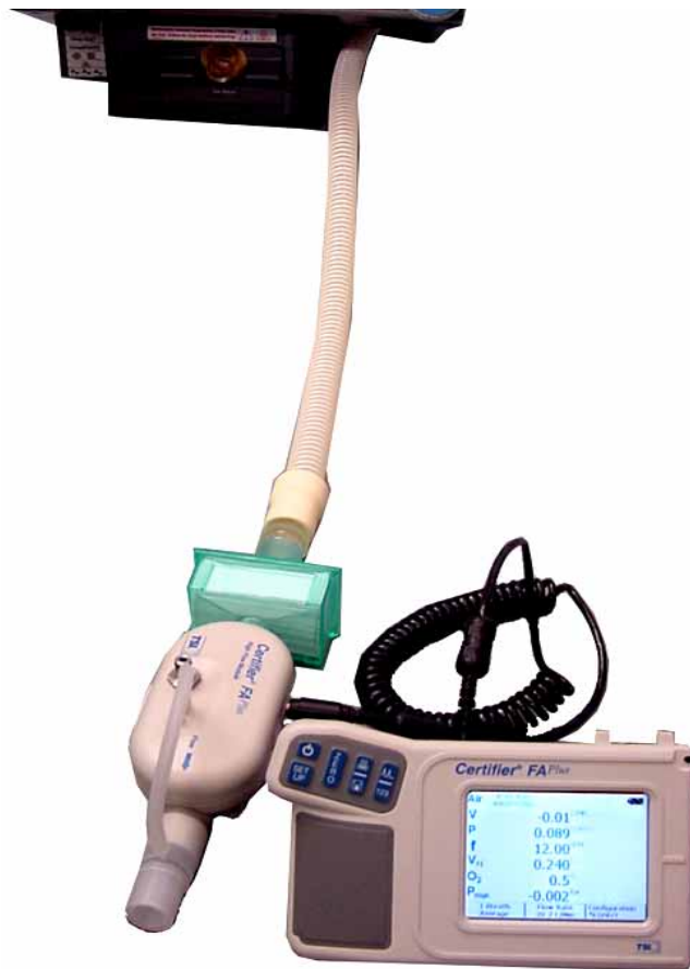
Figure 5-15: Blower Troubleshooting Setup
