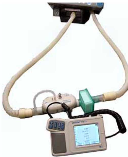
Figure 5-12: Pressure Relief Valve Troubleshooting Setup
