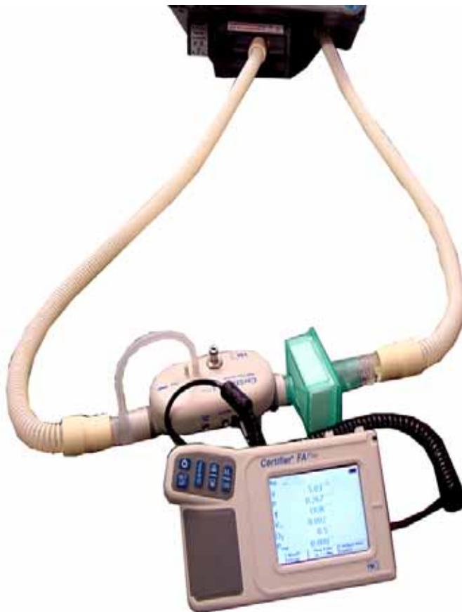
Figure 8-16: Flow Accuracy Test Configuration
