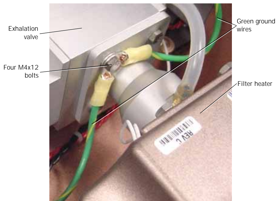
Figure 9-67: Exhalation valve to Filter Heater Connection
