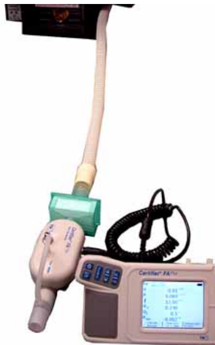
Figure 8-24: Gas Volume Accuracy Test Configuration
