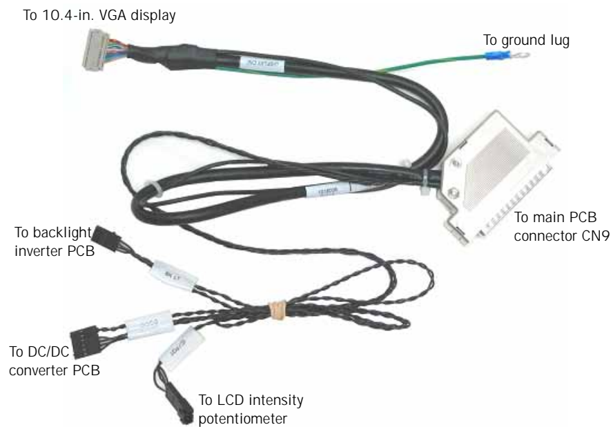
Figure 9-92: Display to Main PCB Wiring Harness
