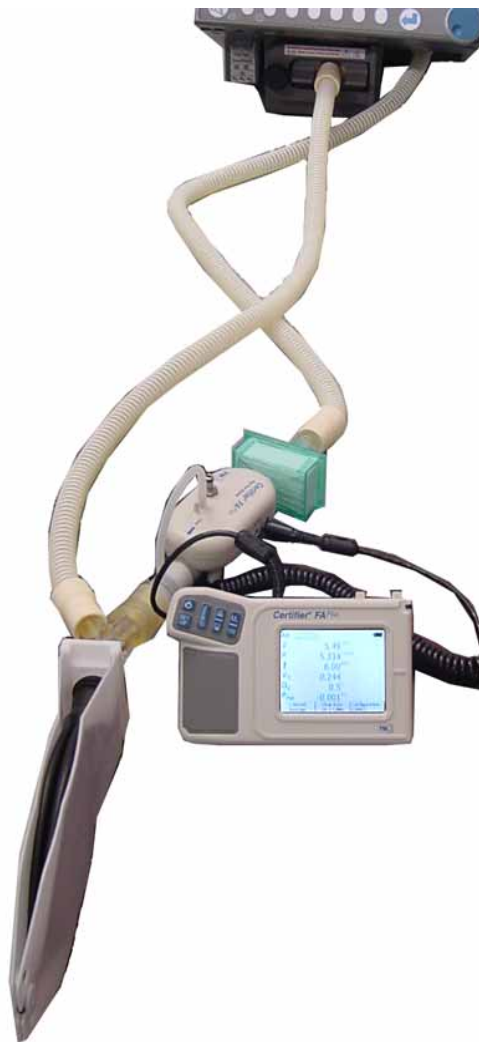
Figure 8-20: PEEP System and Breath Rate Test Setup
