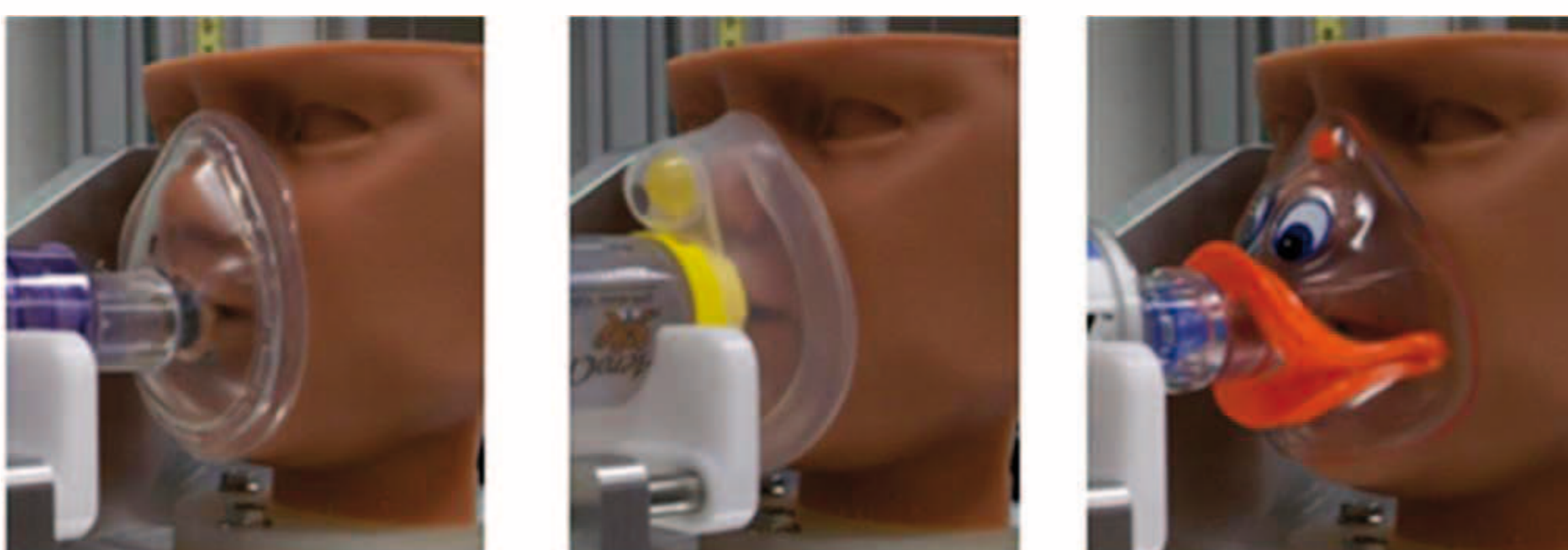
Figure 2. Photos of each VHC-facemask system tested under 0° face replica tilt, 1.9 kg applied force for 1 simulated pediatric breath: (Left) OptiChamber Diamond-LiteTouch, (Middle) AeroChamber Z Stat-ComfortSeal, (Right) Vortex-Spinner Duck.
