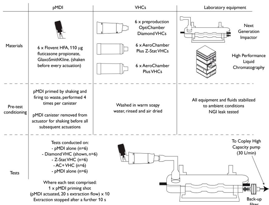
Figure 2. Experimental test method.
