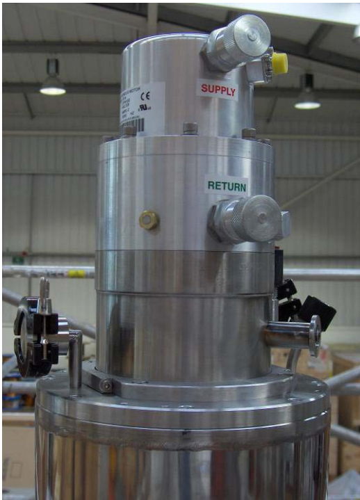
Figure 5 7T magnet coldhead (1 of 2) under vacuum
