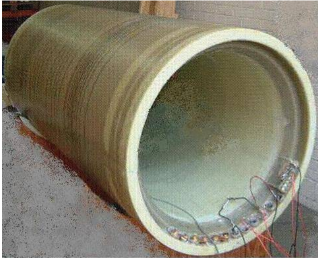
Figure 10 7T Gradient tube. This unit is assembled using lead-free (silver) solder. Illustrated as removed from magnet.
