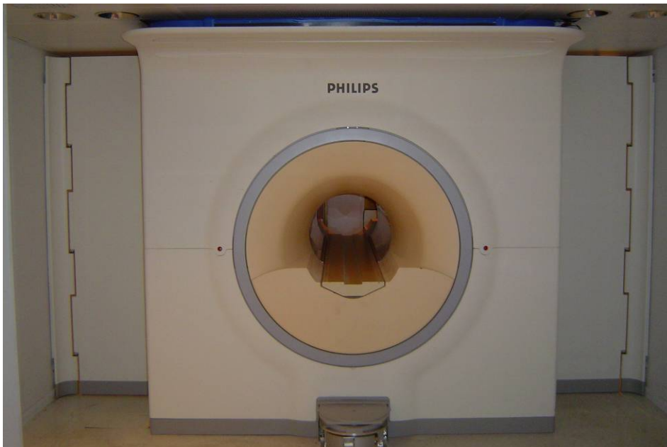
Figure 9 7T front façade, and bore/tunnel liners
