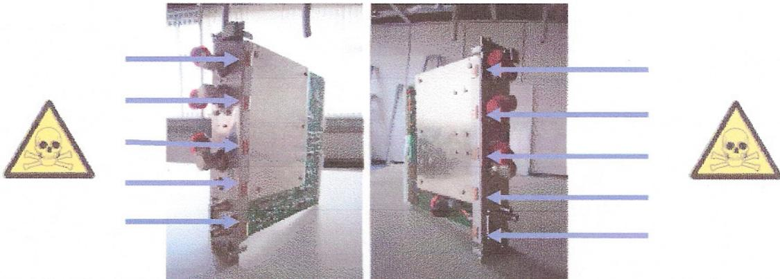
Figure 2, Beryllium Sticky-Fingers on Printed circuit board assembly
